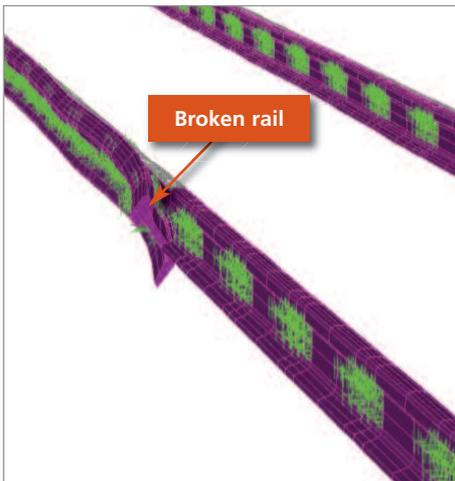
Figure 2 Broken rail simulation
